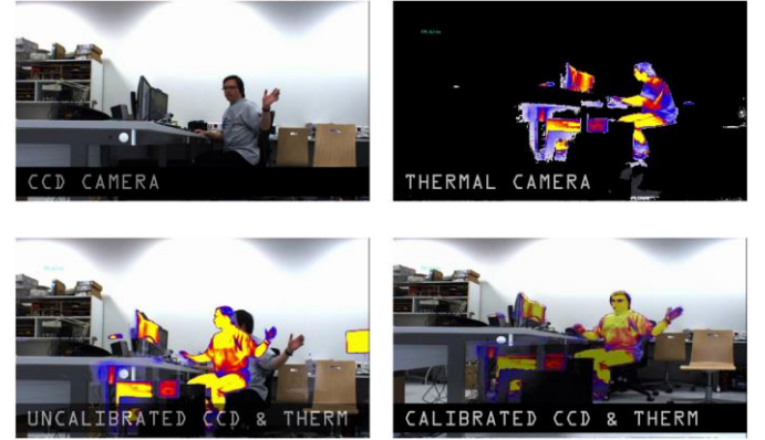
Figure 6. Image of CCD camera (upper left), image of thermal imager (upper right), uncalibrated data fusion (bottom left), calibrated data fusion (bottom right).
