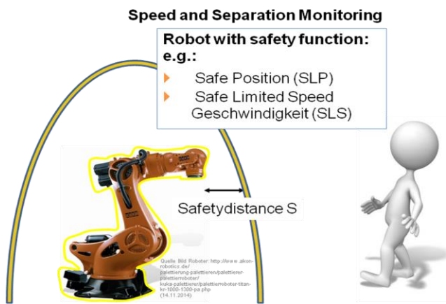
Figure 10. Requirements on the sensor when the robot has safety functions.
