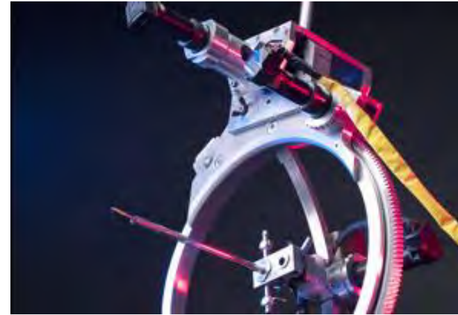
Fig. 5. Complete Software Maintains the Probe Holder Trajectory Pointing at the Target Constantly
