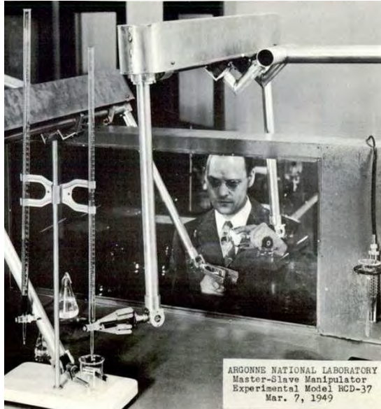
FIGURE 4.—The ANL Model-1 experimental mechanical master-slave manipulator. Motions of the master arm are mechanically communicated to the slave arm. Because the reverse is also true, this is termed a “bilateral” manipulator. (Courtesy of Argonne National Laboratory.)
