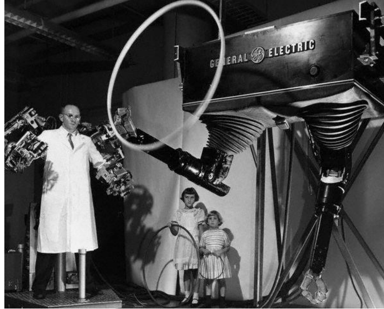
1958/59 Handyman – GE – Ralph Mosher – the first force reflecting manipulator was developed for the atomic aircraft programme
