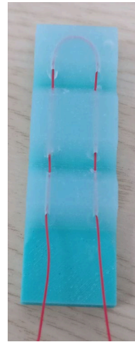
Figure 4. Final produced gripper with cable insert
