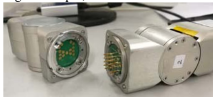
Figure 6 Joint electrical interface design
