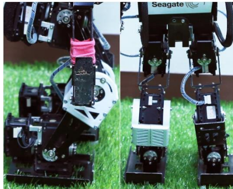
Figure 5. The brace is installed at the right knee of a humanoid robot
