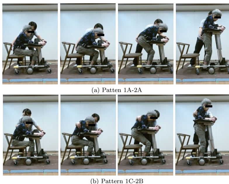
Fig. 5. Standing motion. (a) Suitable motion. (b) Unsuitable motion. In this case, the subject failed to incline her upper body forward so that her COG is over her feet instead of her buttocks in the first phase. The therapists stands near the subject for safety reason and he does not assist the subject during assistance motion.
