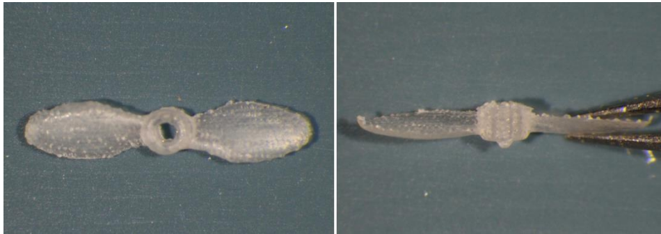
Figure 7. Prototype micro rotor blade
