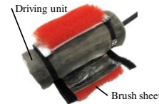
Fig. 8 Appearance of the cleaning unit
