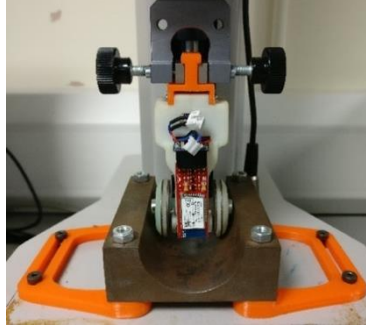
Figure 10: Single column linear force tester with a 10N load cell.
