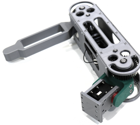
Fig. 7. The final manufactured leg. The initial aluminium parts were manufactured in FDM (PLA base) to reduce weight furthermore.
