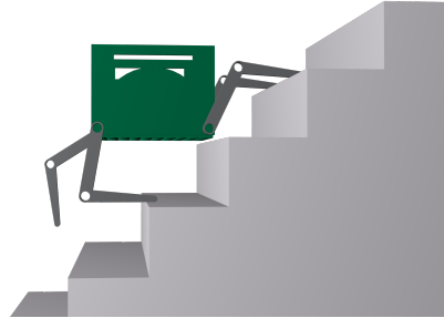
Fig. 5. A highly unfavourable pose: the centre of mass is aligned directly above the footpoints while the lower limb itself is arranged orthogonally.
