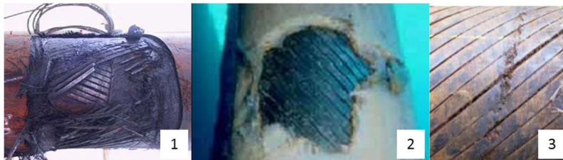
Figure 2. Riser damage: 1) armour wire breakage, 2) external sheath damage, 3) armour corrosion.
