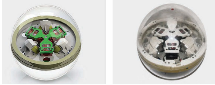
Figure 3. Design of a spherical robot with internal rotors
