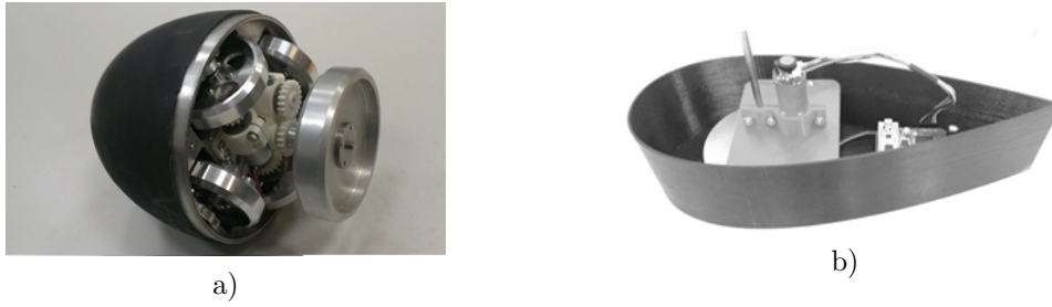
Fig. 1. Propellerless underwater robot without one semi-shell (a). Propellerless aquatic robot with sharp edge (b).
