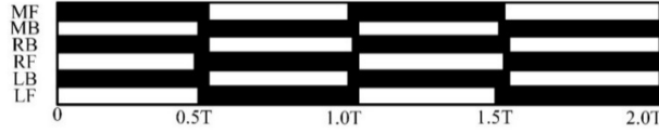
Figure 4. Diagram of gait sequence. Feet in support phase are filled with black and feet in swing are filled with white.
