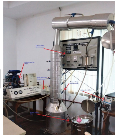
Figure 1(a). Schematic diagram of a Non-Square Pilot Plant Distillation Column.
