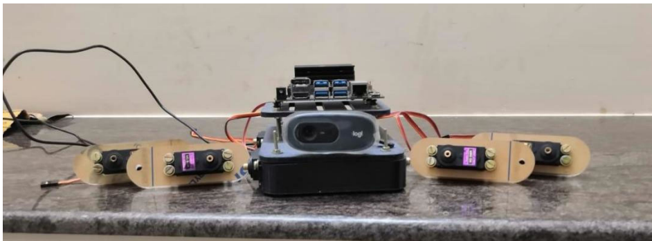
Figure 9. Components of the Prototype before assembly
